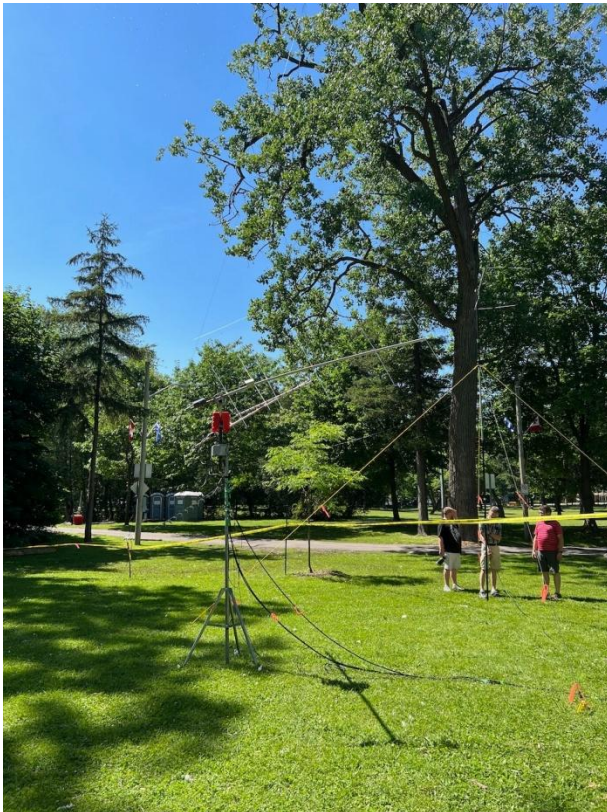
V/U Satellite Antennas on EZ-EL mount © VE2WUP – Patty Micheletti
