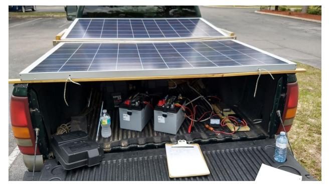
Solar Power charging station used to charge batteries for Alternate Power operations.
