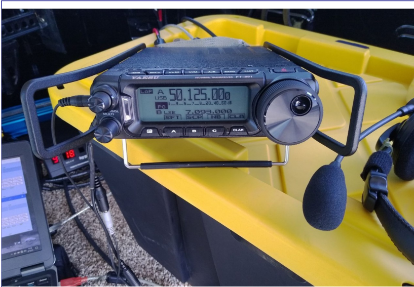
The Yaesu 891 is a great portable radio for POTA or rover contests. With 100 watts on 6 M this was my go to rig for 50 MHz.
