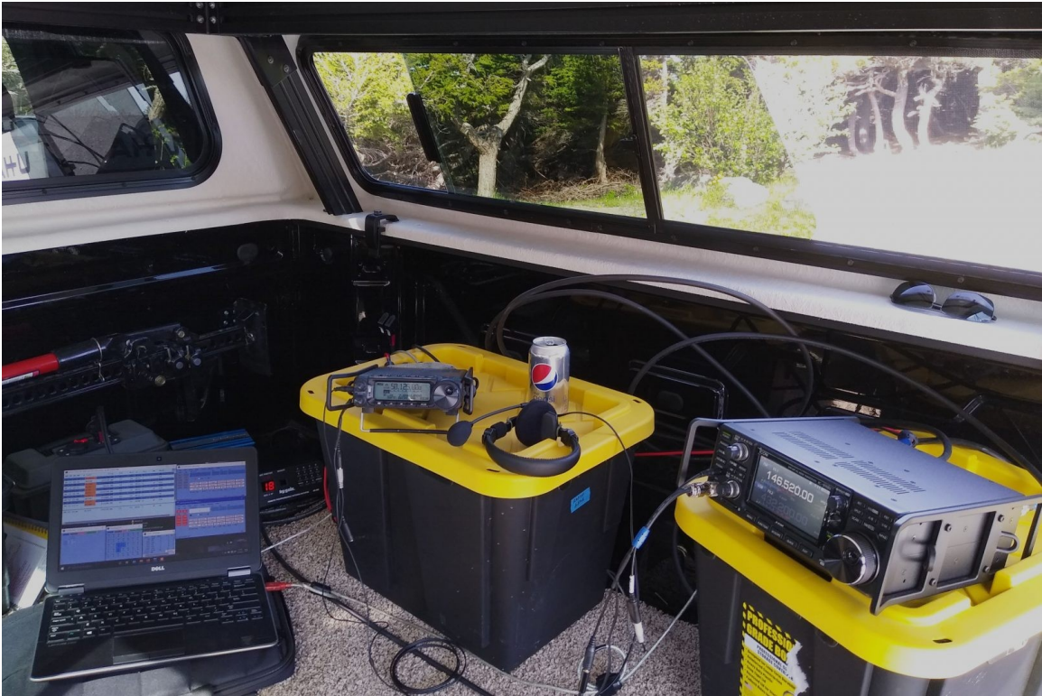
Rover setup in the back of the truck. Power supplies in far corner, logging computer at left, 6 meter rig in center, and VHF/UHF rig at right.
