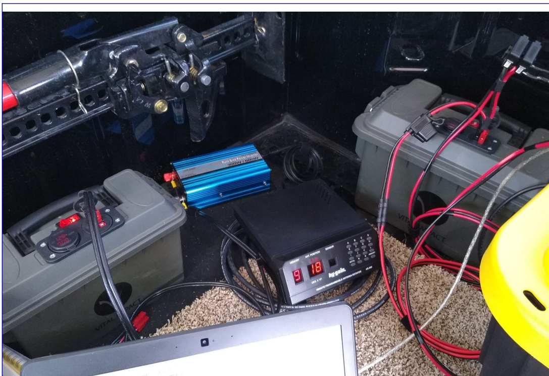
The green ammo cans hold battery packs which recharge from the vehicle while in motion. The blue box is an inverter which powers the black box – a rotator control.
