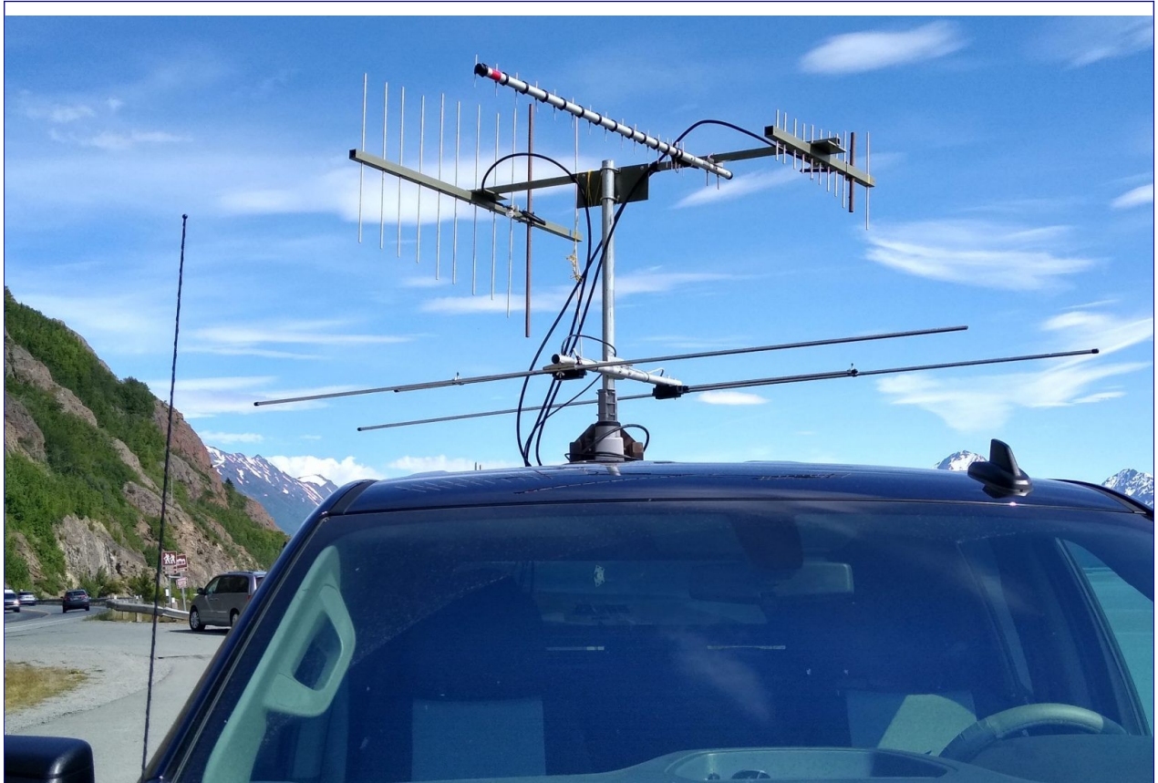
View of the antenna stack set up and in operation. Note that the 2-element 6 meter antenna has to be rotated 90 degrees once I arrive on site. It is too wide to drive down the road with it in operating orientation.
