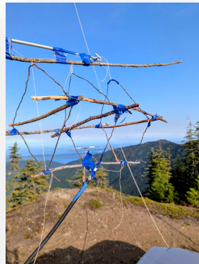
Figure 4 - wire, sticks, and painter's tape last-minute substitute for a left behind 432 MHz long yagi. Best DX 330km.
