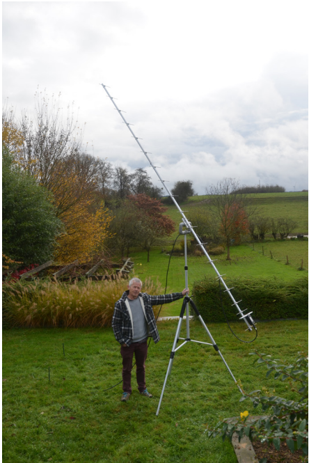
Erik Ickert, ON4PB, participated in the 2024 ARRL International EME Contest using this Yagi fed with 35 W from his Icom IC-7100. It was his first EME contest, and though he only completed two contacts, he said it was a thrill. [Erik Ickert, ON4PB, photo]
