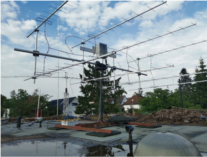
The station of Carsten, DM9EE, sports an 8x11 element 432 MHz array that was given to him by Bernd, DL7APV (SK). It was a prototype for Bernd's 128x11 array. [Carsten-Thomas Dauer, DM9EE, photo]
