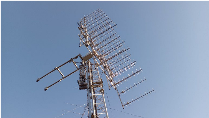
Mila, OK1VUM, used this impressive homebrew 32x9 element array to take first place in the Single Operator, All Mode, 432 MHz category. [Mila Hakr, OK1VUM, photo]
