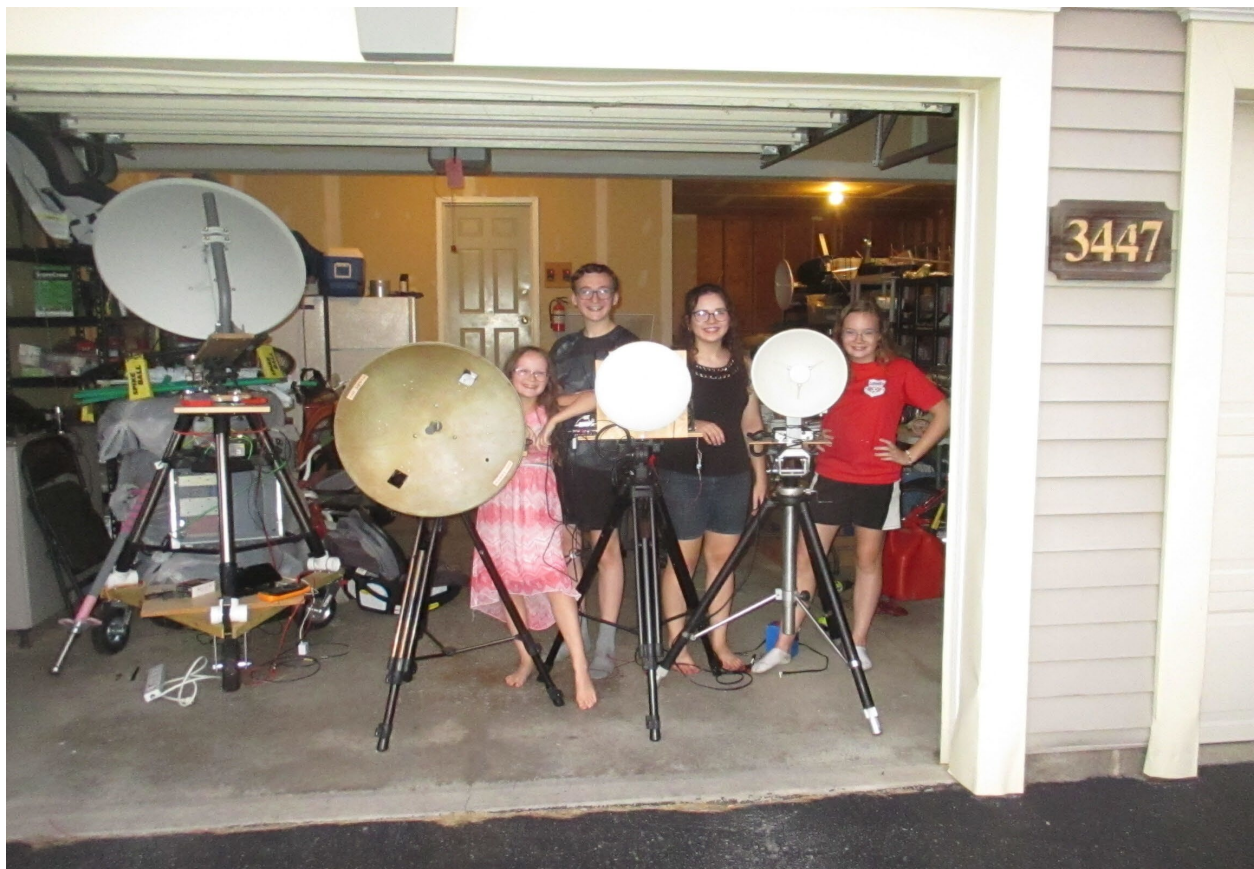
L-R: Maggie, KE2AIZ, Toby, KE2EDK, Alanna, KE2AIY, and Dora, KE2AJA. Equipment L-R: 20 W 10 GHz station, 3 W 10 GHz station, 47 GHz station, 76 GHz station (borrowed from KB8VAO for the contest). (24 GHz Wavelab system not pictured.) ( KØSM, photo )
