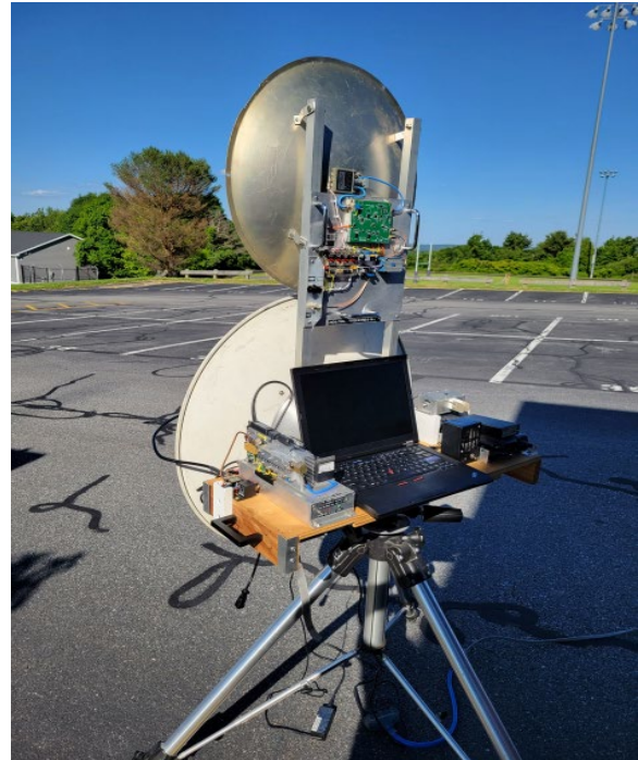
Fred, K1FMS, added 24 GHz to his 10 GHz system for 2024. The top dish is for 24 GHz and netted Fred 25 QSOs on 24 GHz. Read more about his efforts to get more stations on 24 GHz in his sidebar. ( K1FMS photo )
