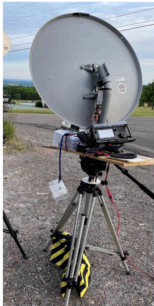
A view on a dry day from K2UA's operating location for the September contest, showing his 10 and 24 GHz dual-band setup. The antenna was a 76-cm Winegard dish fed by a W1GHZ dual-band feed. The plastic container hanging to the left is used to protect the feed, T/R relays, and low-noise receive amplifiers during travel. (Photo Courtesy Rus Healy, K2UA)
