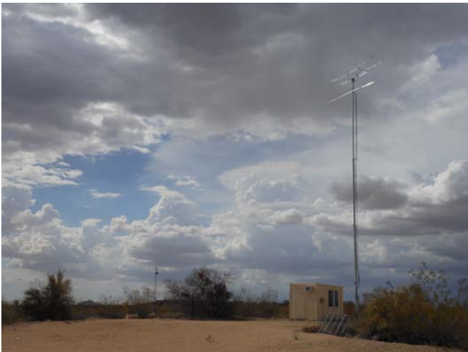
The WO1S Unlimited Multi shack in DM34oa with a long-boom 2-Meter Yagi and a two-antenna 23cm array. [John Kountz, WO1S, photo]
