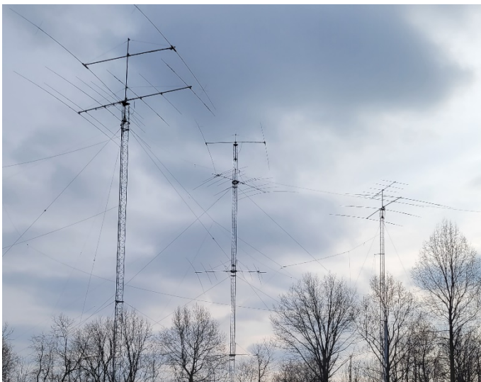
Flexible multi-band arrays like this one take the guesswork out of making two band sequentially interleaved QSOs. [Bud Trench, AA3B, photo]
