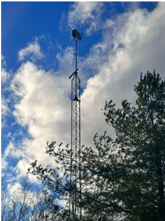
W8BYA's home station antenna setup for 10 GHz, with a tower-mounted 2-W transverter just behind the dish. (W8BYA photo)
