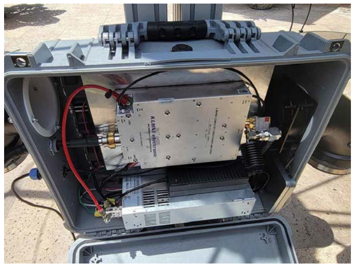
KB2SA: 1200W Kuhne PA (for 1296-ed.) located near dish in a Pelican case. [Bill Siino, KB2SA, photo]
