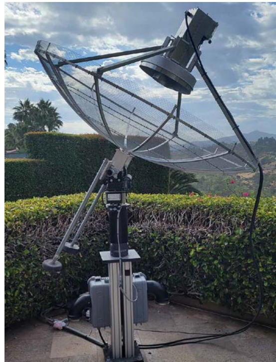
KB2SA's 1.9m f/d=0.35 mesh dish (for 1296 MHz -ed.). 850w into RA3AQ (2008) feed with custom tuned choke. [Bill Siino, KB2SA, photo]
