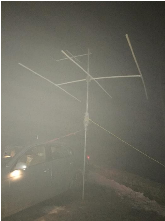
Six- and two-meter antennas icing up at AK4U. High winds, bitter cold, fog, antenna icing, and dead bands from location at Knob Hill VA created a challenge and had Paul looking forward to June. Oh yes, propagation was flat to non-existent. (photo by AK4U)
