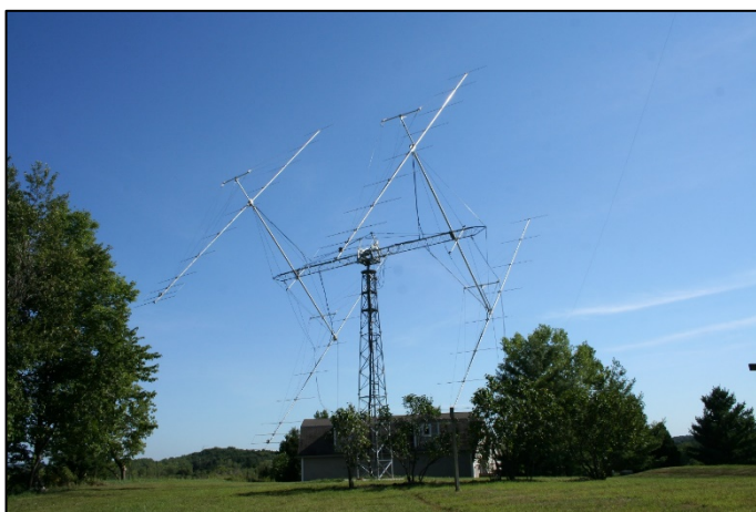
The 4x10 element 6-meter LFA array of Dave, KJ9I allowed him to work a number of small 6-meter stations. [Dave Schmocker, KJ9I, photo]
