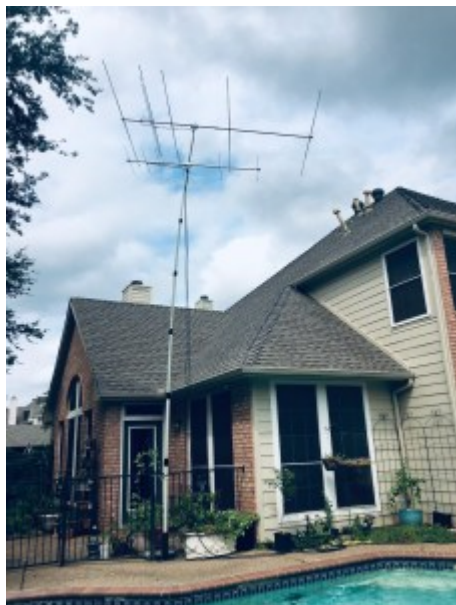
K5ND backyard push-up mast with 6- and 2-meter Yagis, [Jim Wilson, K5ND, photo]
