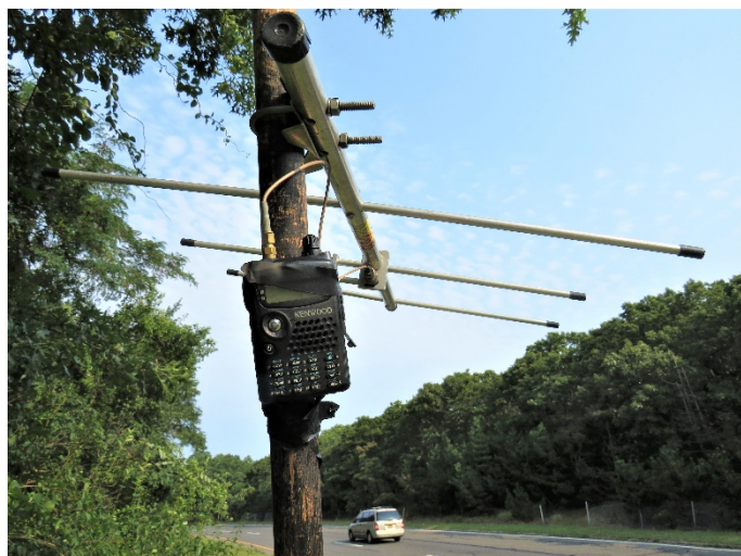
Here is the WB2AMU 222 3-element beam on a stick pointed towards FN42 in Massachusetts from FN30, Central Long Island, NY. Not much feedline loss and good for 8 QSO's and 3 grids, including K1KG in FN42. [Ken Neubeck, WB2AMU, photo]
