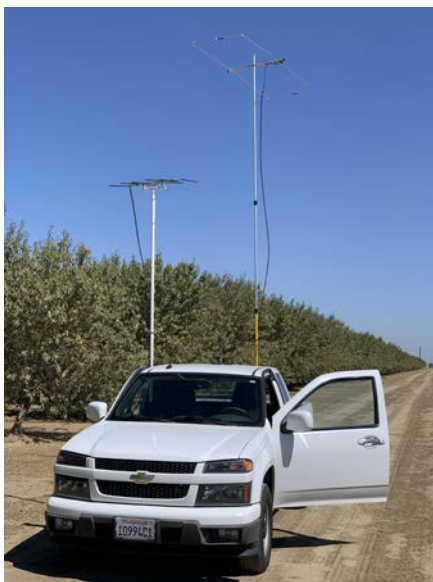
KG6BXW/R, Limited Rover setting up in CM96 with a 6-meter Moxon and Elk LPDA [Kyle Hamilton, KG6BXW, photo]
