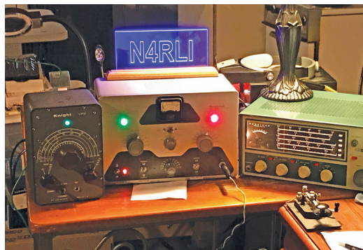
For SKN 2021, Ralph Irons, N4RLI, uncovered his vintage station, consisting of a Heathkit DX-20 transmitter paired with an Allied Radio Knight-Kit V44 VFO, and a Heathkit HR-10 receiver. [Ralph Irons, N4RLI, photo]
