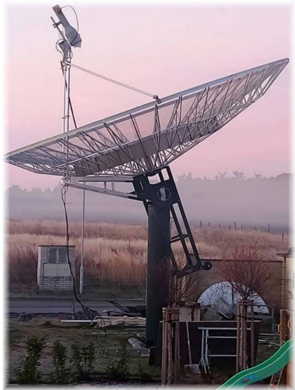
OK1DFC used his latest homebrew 8.5m offset dish to log 76 QSOs on 1296 MHz EME [OK1DFC photo]
