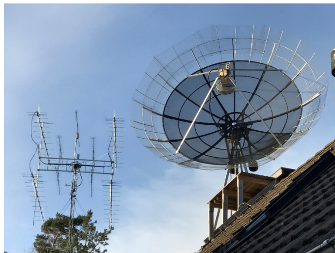
This array of Yagis and a 3.8m dish at SM4GGC enabled 170 EME contacts for the contest. [SM4GGC photo]
