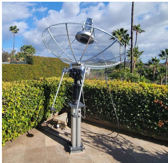
KB2SA uses this 1.9m f/D .35 mesh wire dish with a septum feed and scalar ring effectively on 1296 [KB2SA photo]
