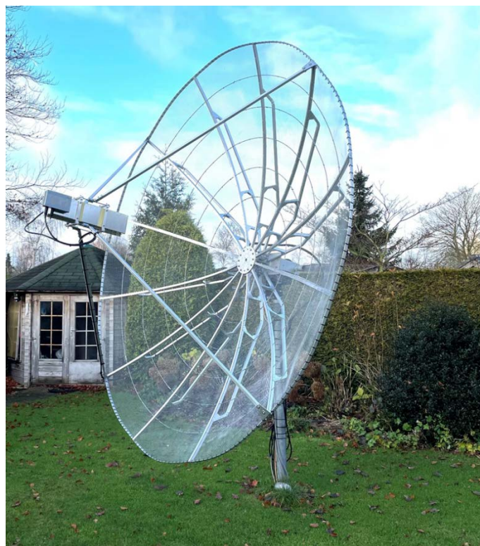
PAØTBR homebrewed this 3.5m dish and with only 3 watts at the feed was able to make 13 QSOs on 1296 MHz [PAØTBR photo]
