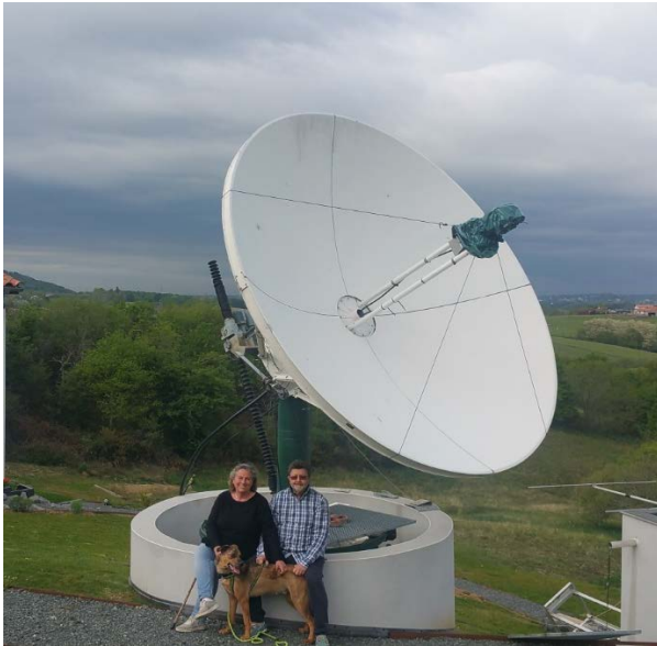
F2CT and family with his 3.7m solid dish used on 1296 MHz and 10 GHz in this year's contest [F2CT photo]
