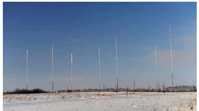
The 160-Meter 4 square antenna system of Nikolay, RM4F secured him a top-ten finish. [RM4F, photo]
