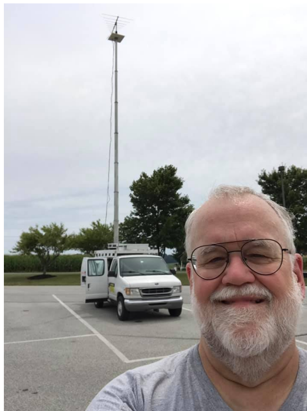
Pete, KØBAK, operated using a 2m-23cm log periodic antenna and a new Q5 5-band transverter from his repurposed ENG news van. [Peter Kobak, KØBAK, photo]
