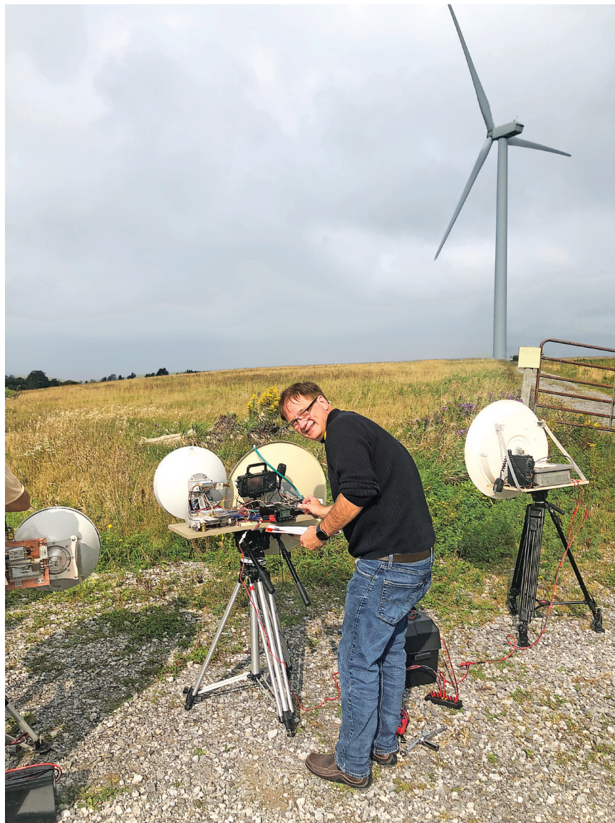
Bill Rogers, K2TER, operated his new 10 and 24 GHz microwave gear in the 2021 ARRL 10 GHz and Up Contest. His best DX for the event was a pair of 445-kilometer 10 GHz contacts with Dale Clement, AF1T, and Mickie Clement, W1MKY, on Martha's Vineyard in Massachusetts. [Chris Shalvoy, K2CS, photo]
