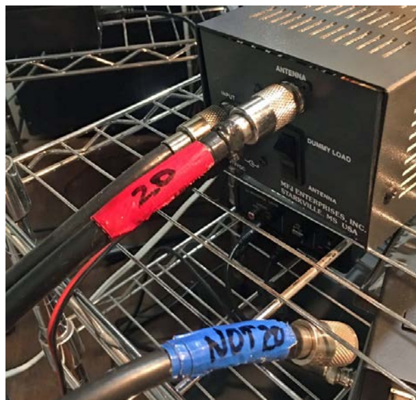
K5TA's simple, inexpensive, and ultra-reliable antenna switching system. (K5TA photo)
