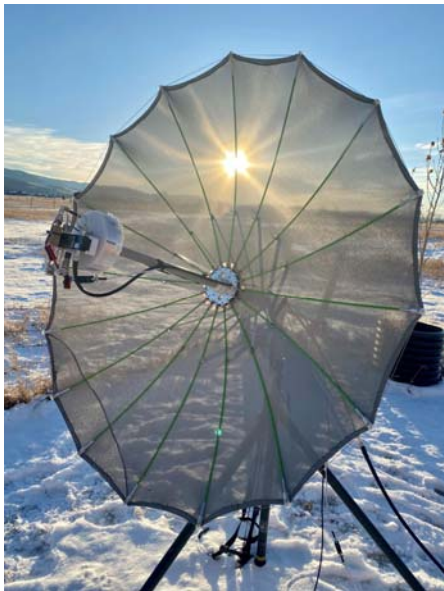
Gene, KB7Q was able to work 29 JT65 QSOs on 1296MHz with this 1.6m foldable metalized fabric dish, circular patch feed and 275W. "It was fun being the Montana multiplier!" The dishes are custom made by Paul W2HRO and come in sizes up to 2.4m [Gene Shea, KB7Q, photo]
