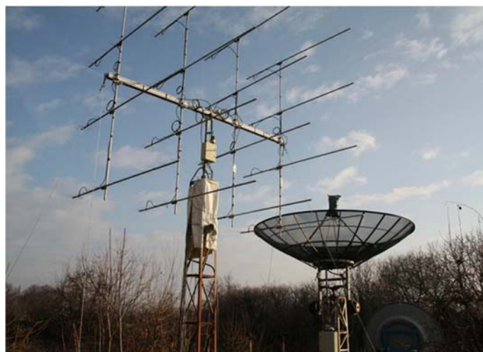
Ned, LZ1DX shows his Yagis and dish for his 144 MHz, 432 MHz and 1.2 GHz three band contest effort [Ned Zaprianov, LZ1DX, photo]
