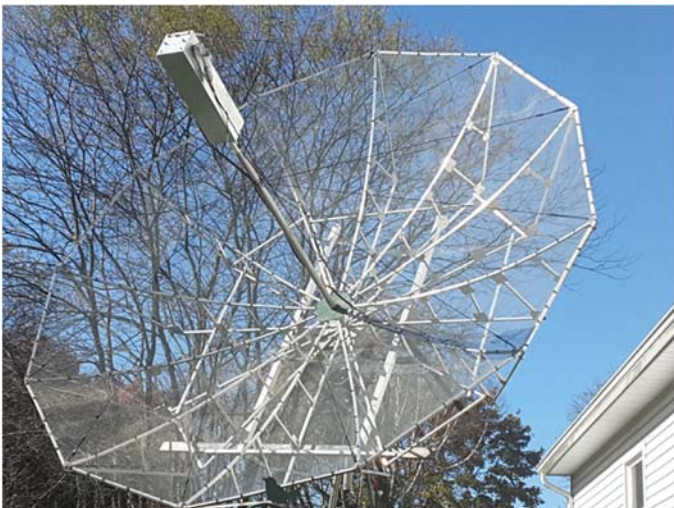
Skip, W1PV uses this 3.6m dish on 1296MHz with multiple guys on the feed strut. The same dish is used for 432MHz with another feed. [“Skip” Paulsen, W1PV, photo]
