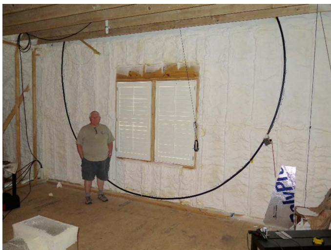
Barry, K6RM, stands beside the 15-foot-diameter magnetic loop transmitting antenna he used for the contest. Built out of 7/8” Heliax®, it is 25 feet above ground in his attic. [Barry Pfeil, K6RM, photo]
