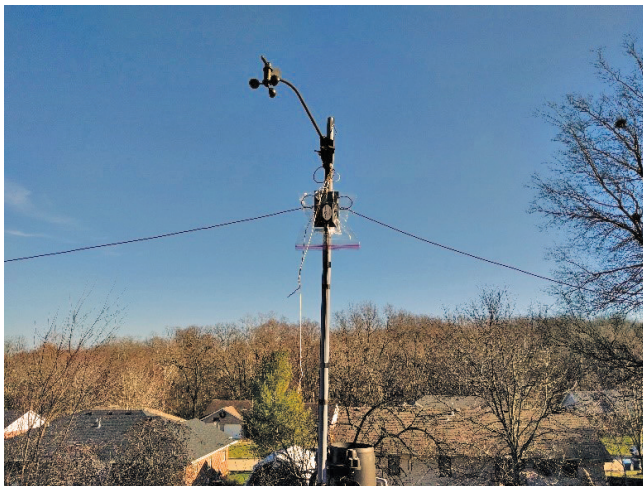
It doesn't take a large antenna to operate the ARRL 10-Meter Contest. Tim Raymer, KA0OUV, operating as N0SS, used a dipole antenna mounted above his deck, with a high-tech weatherproof balun enclosure. [Tim Raymer, KA0OUV, photo]
