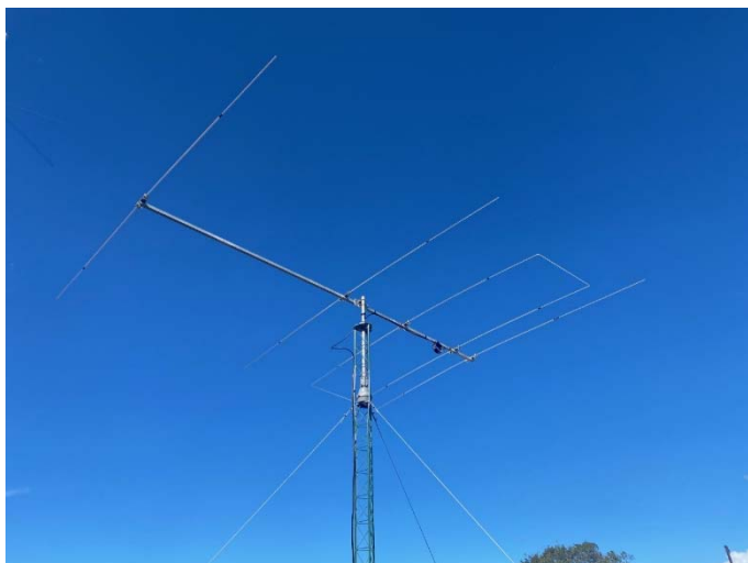
Photo 3 – Charlie, TI2CDA, built this good looking 4 element Loop Fed Array antenna just in time for the contest. He made almost 500 contacts with it! [Charlie Azofeifa, TI2CDA, photo]
