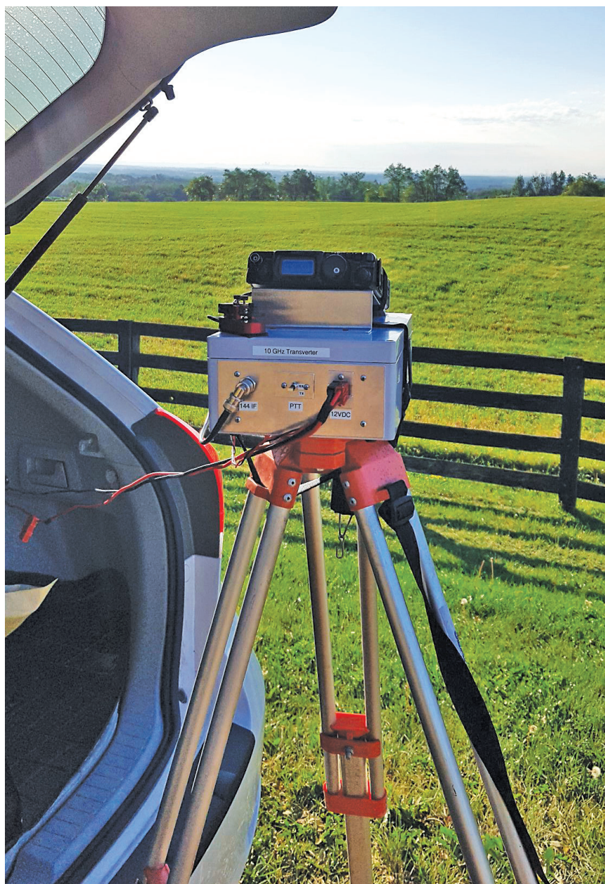
Andrew Mitchell, VA3CW, enjoyed his first microwave contest during the 2020 ARRL 10 GHz and Up Contest. He set up his 10 mW transverter in grid square FN03, and completed two 10 GHz contacts with Andrew Flowers, K0SM, in grid square FN12 — a 219-kilometer path. [Andrew Mitchell, VA3CW, photo]
