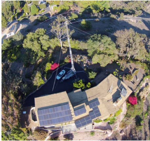
A drone's view of the NX6T multi-op high-power station. The antennas were held aloft by a couple trailer-mounted towers, and included a 2-el 40 meter yagi, 3-el SteppIR, F12 tribander, and an 80 meter dipole. (Photo from Dennis Vernacchia, N6KI).
