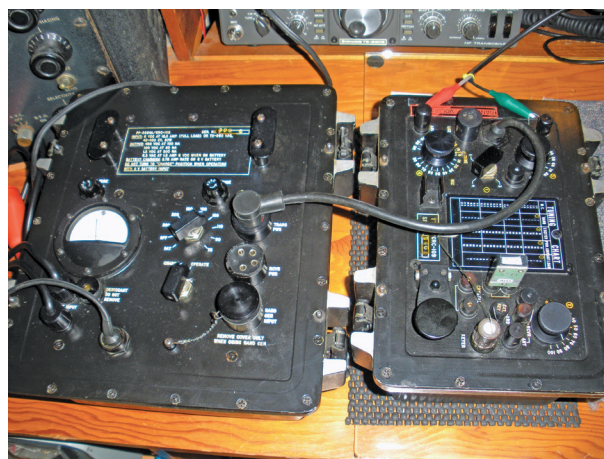
Joe, KA4WJB, made four contacts using this T-784A. This unit (later designated GRC-109) first appeared during the Cold War and was intended for use by CIA agents. Joe said, "The rig even has a built-in key." [Joseph Scoglio, KA4WJB, photo]
