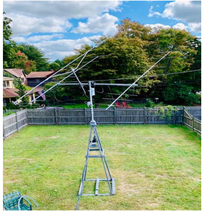
William Corbin, W3CJK's homemade wooden tower with antennas for 2 Meters, 432 MHz, and 1.2 GHz. (William Corbin, W3CJK, photo).
