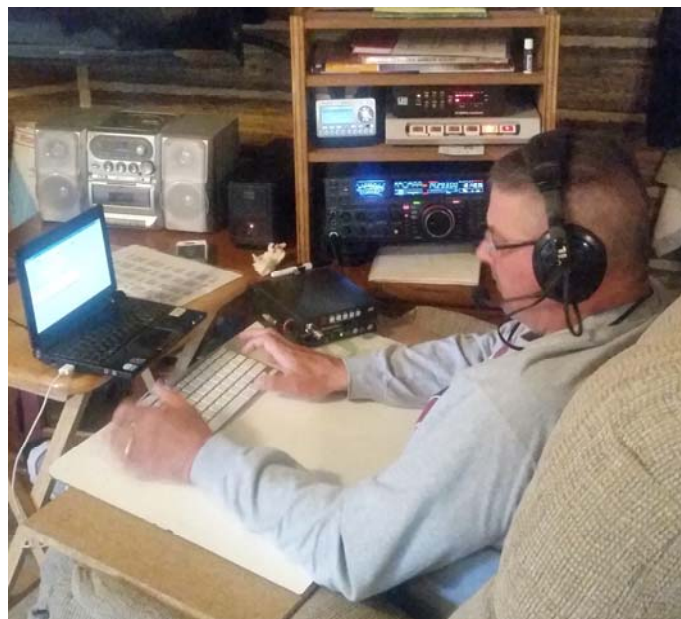
KK7AC, SOULP 3 rd place. Andy says "The set-up is quite humble at the summer cabin; transceiver, voice keyer, and automatic tuner. The contest cabin has the most important elements of a good station: Location (hilltop with 360° take-off), antennas (high), noise (none). Over time, I have dialed in my makeshift contest "desk" that sits on my lap that I formed out of a dry erase board so I can quickly make notes or calls then erase later. I have also found, for me, a recliner provides hours of comfort for those long in chair runs. I transform the living room into the contest station with a fireplace in front of me and a view of the beautiful outdoors." (Photo courtesy of Andy Smith, KK7AC.)
