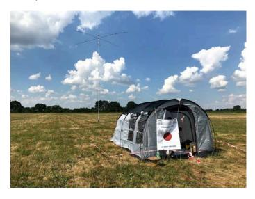
All WRTC 2018 stations had the same antennas on equal terrain. Each boasted a rotatable Spiderbeam for 20-10 meters, a 40 meter dipole along the tribander's boom and a fixed 80 meter dipole. (photo courtesy of 9M6NA)
