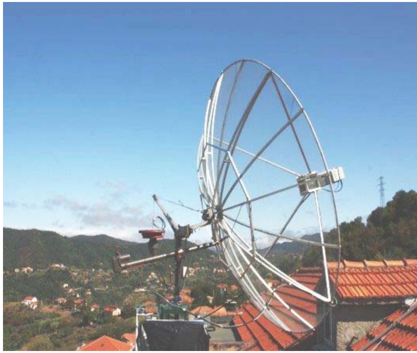
Valter, IK1FJI, used this 3.2m dish on his roof to make 60 CW QSOs on 1296 MHz despite strong winds. [Walter Dolso, IK1FJI, photo]
