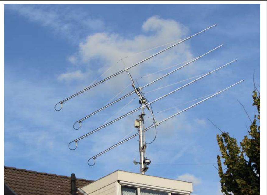
Peter, PA2V, was able to work several 1-Yagi stations using this 432 MHz 4-Yagi array. [Peter Gouweleeuw, PA2V, photo]
