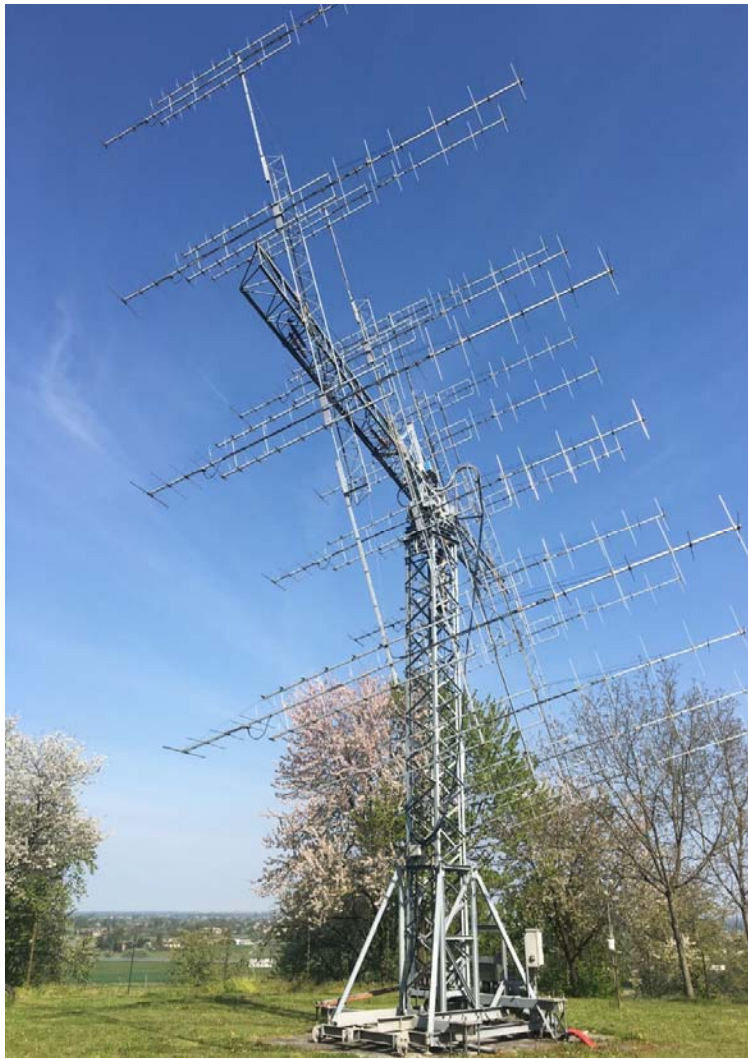
I2FAK's 144 MHz array: 16x19-element Log-Loop-Yagis in H plane, plus 16x6-element Yagis in V plane, with adaptive polarization on Receive. [Franco Giorgi, I2FAK, photo]
