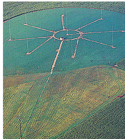
The K9DX ultimate nine-element 160-meter array is no longer in place, but it remains a dream of many hams. Read more about it at https://nidxa.org/memberWWW/k9dx_antennas.htm , or its related presentation from the 2008 Dayton Hamvention Contest Forum, available at https://www.kkn.net/dayton2008/contesting_with_28_miles_of_feedline . [NIDXA and K9DX, photo]
