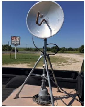
WA5YWC three-foot prime focus dish mounted on bed of truck. (Photo provided by Al Ward, W5LUA)
