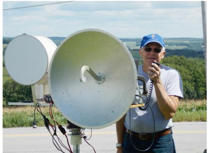
David, K2DH, operates from west of Rochester, NY at FN02xu. His setup runs 10 watts to his 10 GHz dish and 2 watts to his 24 GHz dish. (Photo K2DH)
