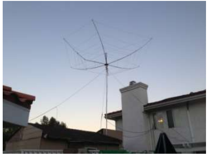
The Hex-Beam at NC6K did yeoman’s duty on the higher bands. (NC6K Photo)
