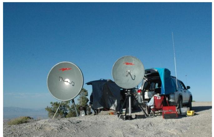
"Camp" on top of Mt Potosi, Nevada. Las Vegas is behind the dishes. On the left is Robin, WA6CDR's 6-foot dish where he runs 10 watts. On the right is Mel, WA6JBD's 4-foot dish which he illuminates with 30 watts. (Photo by WA6CDR)
