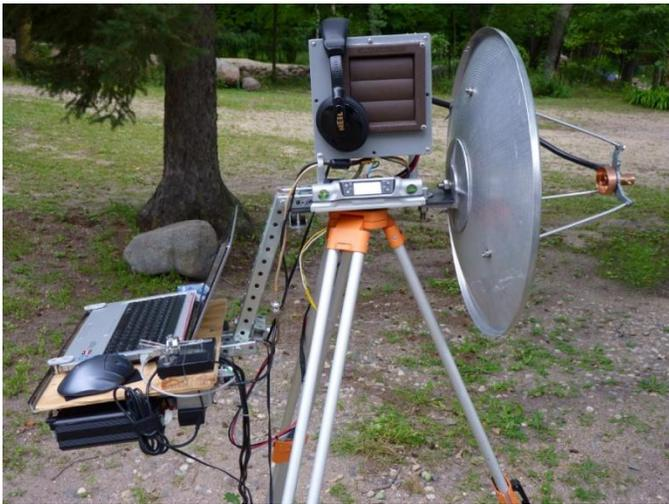
Check out Jim, KØMHC's tripod setup that includes laptop and SDR. His neat integration takes 10 GHz portable activity to the next level—involving SDR in his operation. (Photo by KØMHC)
