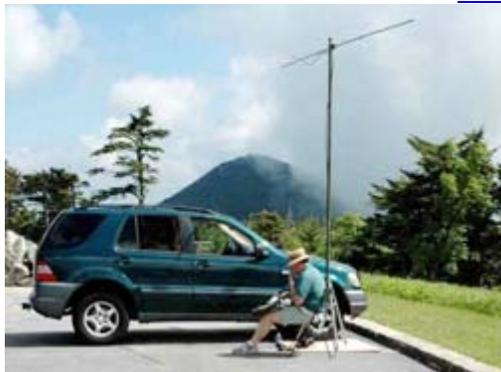
KB5YZG on his first VHF outing using an ICOM-706, with an 11 element yagi on top of a stack of fiberglass tent poles. Car battery provided talk power, elbow provided rotor power.
