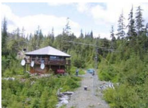
The KL7FF QTH - The 2-meter 12-element Yagi can be seen mounted on the mast on the deck to the left side of the cabin. The 6-meter 8-element Yagi can be seen in the right foreground, mounted on 3 tower sections. The 2-meter station ran 400 watts output and the 6-meter station ran 600 watts output.
