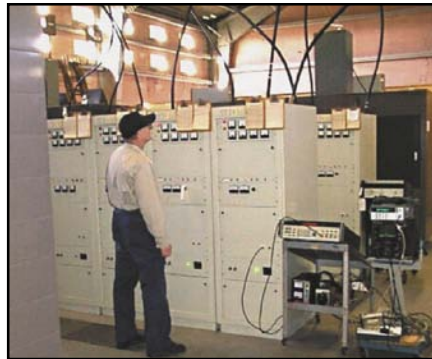
Steve, WB6UZX, in front of the Henry transmitters for 14 and 7 MHz used at the K6KPH site for the West Coast transmission of the W1AW Field Day bulletin. Also shown are the signal generators and frequency counter, and in the back row the Henry for 21 MHz. Be sure to see the complete story on the Web at www.arrl.org/contests/results and look for Field Day 2004.
