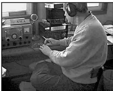
National Contest Journal Editor Carl, K9LA, used an old Ranger II and Drake 2B (his General station back in the early '60s) with a J-38 key.
