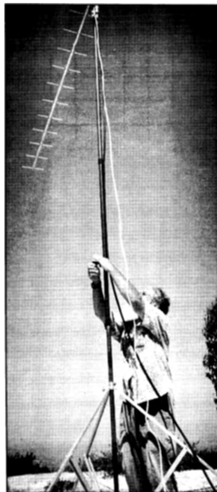
John, KE6GFF, sets up his backpack antenna for the contest. He uses a most unusual mast made out of three sections of graphite fiber all held together with Velcro.
