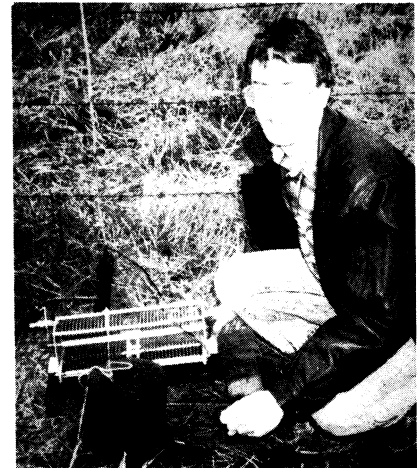
Jon Jones, NO0Y, tunes the series capacitor on his shunt-fed vertical.
