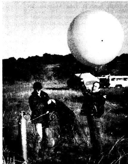
WB5AZI (l) and WA5MWD launch multioperator-station WA5MWD's balloon-supported 1/4-wave vertical antenna.
