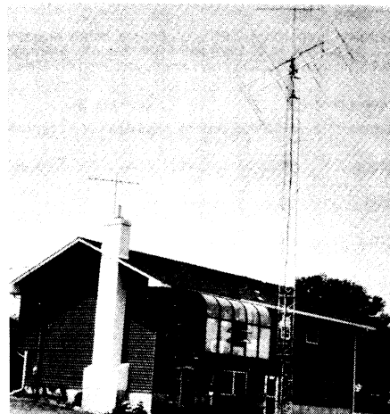
WB3ESS, submitted a single-band 432 score from EPA. John uses a homebrew transverter on 432 to his TS-830S. John's skyhooks include eight KLM 16-element beams on 432 at 50 feet, an 8-element quagi on 220 MHz and a single 12-element KLM beam on 2 meters.
