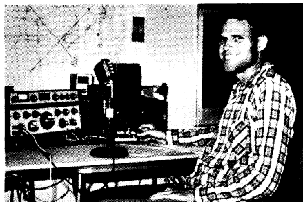
That Signal/One, CX-7 and Hallicrafters HA-2 Transverter feed a KLM 13-element, long-boom antenna. Howard, WA3EOQ, does 2 meters for K3LNZ/8 — number-one multiop station from West Virginia.
