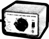
**Antenna Noise Bridge** (an-ten-a noiz brij), n. Omega-t's name for a specialized testing device that checks your antenna system for resonant frequency and coaxial impedance.
