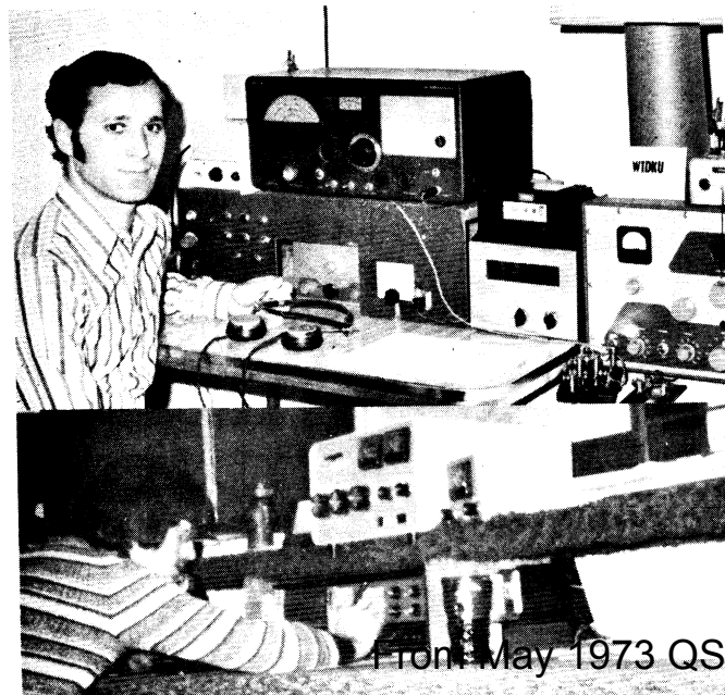
Below top: Using a DX-100, S-40 and R4 with a multiband vertical and 2 element 20 meter beam radiators W1DKU ran up a very nice 69K low power cw score to take the Western Mass. section certificate. Below, bottom: Participating in his first SS since his Novice years in 1966 WA0TKJ walked off with the section award in Kansas. A tribander and dipoles at 50 feet spewed his signals through the country for the tune of over 158K. Right: Some of the antennas of Mo. Section leader W0TDR. The 2 element 40 meter beam on top is at 75 feet. The lower beam is a 4 element 20 meter radiator. Warren has another tower that supports a 4 element 10/15 quad at 62 feet. These antennas can be fed by either of 2 S-lines followed by a choice of a L-4 or SB-220 afterburner. Not bad, eh?
