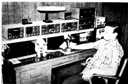
Central-Division single-op champ (by a fat margin) K9KFR fondly regards his HS-type cat and perhaps ruefully considers the QSOs he missed on 2 because the kw amplifier expired. Bob's metalwork helped: for 6, it was 11 elements at 90 feet; for 2, how about 15 elements up 105 feet.
