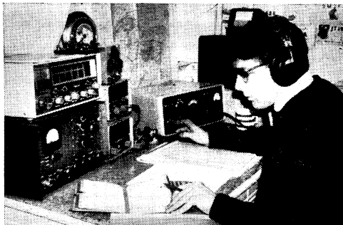
K4GSU/3 found the going tough in Maryland and looks forward to a return to Kentucky! Bill's winning 118-K c.w. effort led a difficult section. Gear shown includes an HT-46, homebrew pair of 6146A's, Handbook Keyer, T-O Keyer v.f.o. and 75S3-B.
