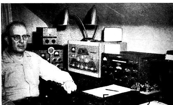
W8OYI has been a ham since '26 and has always been a "regular" in the SS. Joel used a Viking I on 10 and 15 and the DX 100 on 20-40-80, with 75A-4 receiver. A mighty fine code showing, top W8 with 1005 two-ways.
